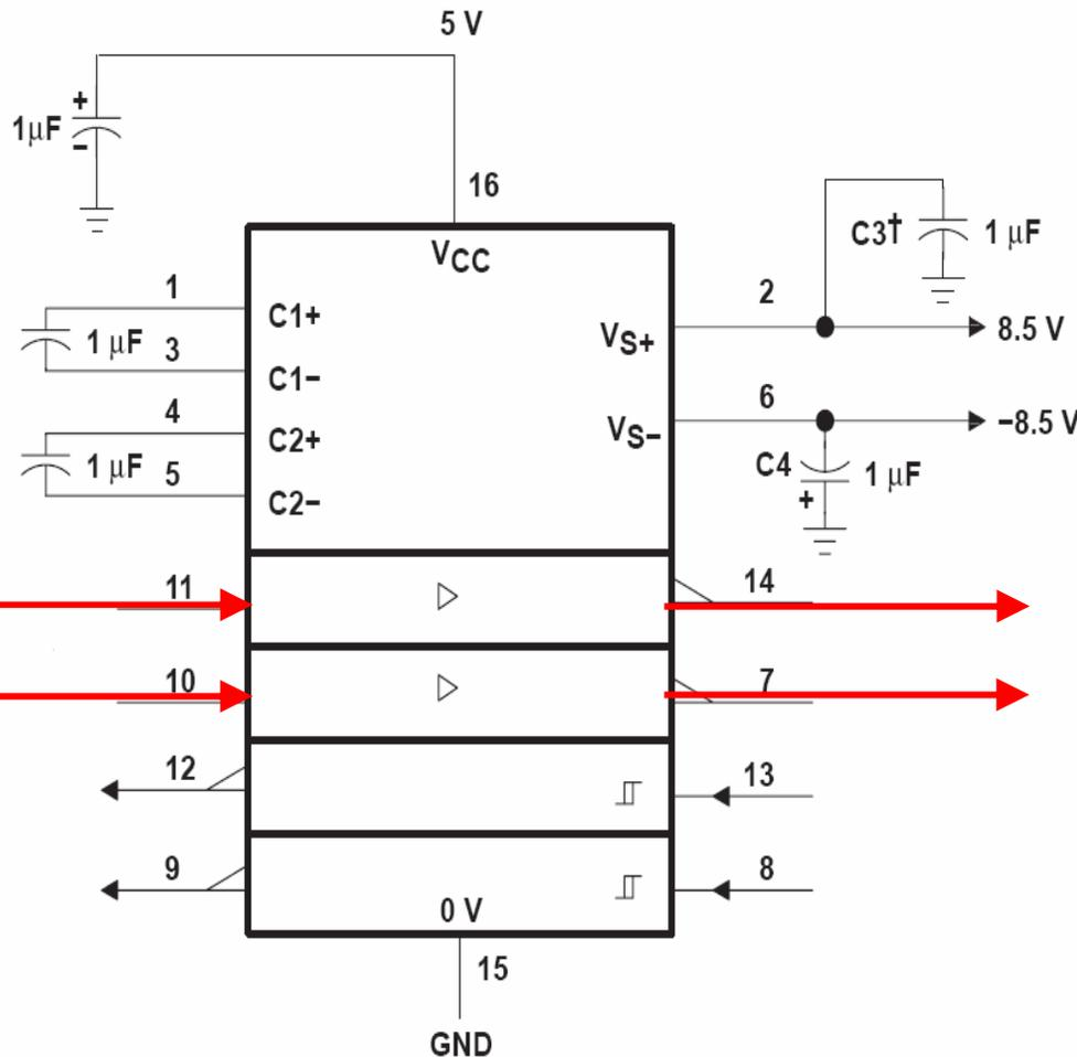
Levels of information are converted to the new voltage values to meet the RS232 protocol
