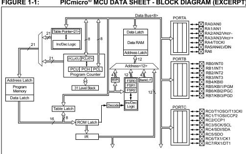
PICmicro® MCU DATA SHEET - BLOCK DIAGRAM (EXCERPT) FIGURE 1-1:
